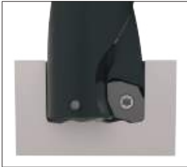
Periphery edge chip formation:
