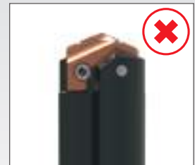
Standard Series Insert + Half Series Holder
