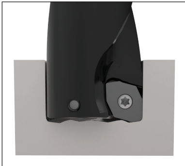
Periphery edge chip formation:
